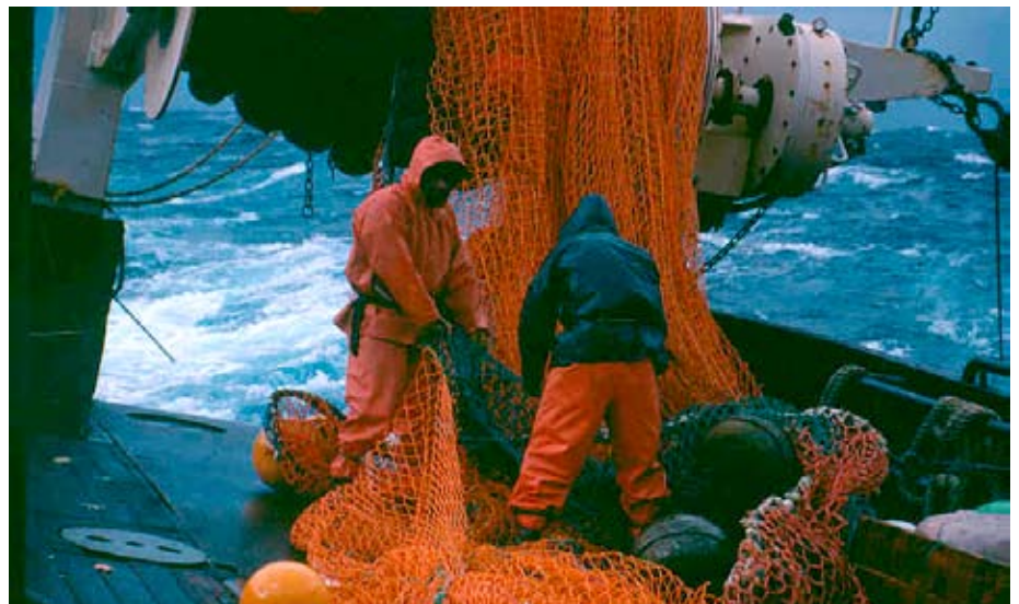
Deck hands tying off a Codend on a trawler harvesting Atka Mackerel in the Aleutian Islands
